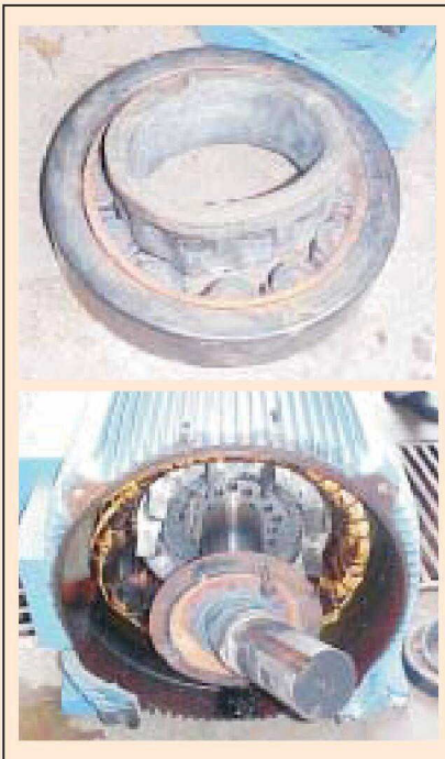
Figure 6 - Detail of damage of rolling bearing and shaft because of high temperature condition.
