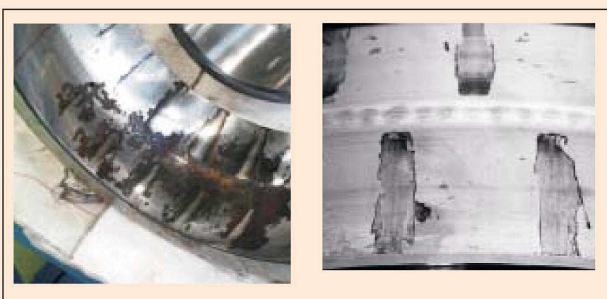
Figure 2 - Detail of rolling bearing raceways with corrosion from water contamination.
