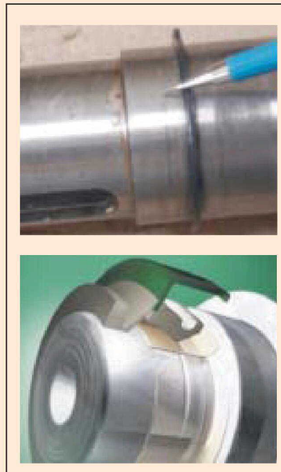
Figure 10 - Example of shaft wear on the contact with shaft seal lip. The scheme of mounting of wear sleeve is also shown.
