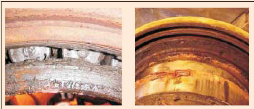
Figure 1 - Detail of rolling bearing with degraded grease because of water contamination.
