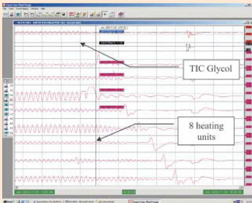
Figure 2. Aggressive tuning in a temperature loop caused oscillations in several other loops. By means of the suitable loop tuning it was possible to eliminate the oscillations (Emond et. al , 2004).
