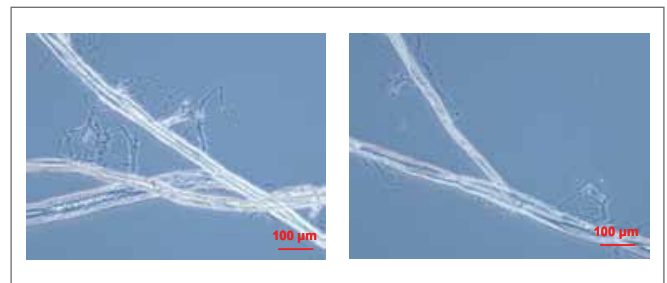
Figure 9. Pulp in the H + -form refined at 125 kWh/t. Fines had been removed. WRV was 1.79 when the fines were present in the pulp sample
