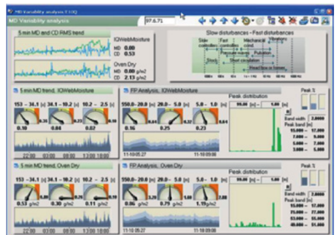
Figure 13. Papermaker’s variability “dashboard” from a Finnish board machine
