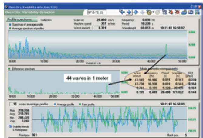
Figure 10. Spectral difference reveals a fast MD cycle from scanning data
