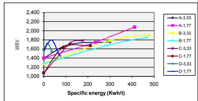
**Figure 5.** Water retention value (WRV) versus specific energy of refining
