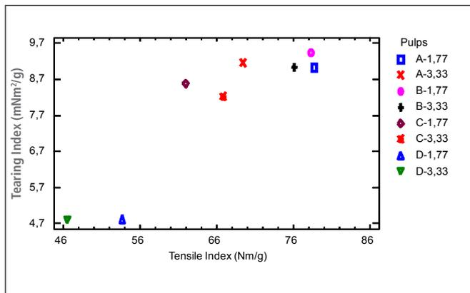
**Figure 6.** Tear Index versus Tensile Index of the repulped papers of density  $0.75 \text{ g/cm}^3$  for both refining intensities
