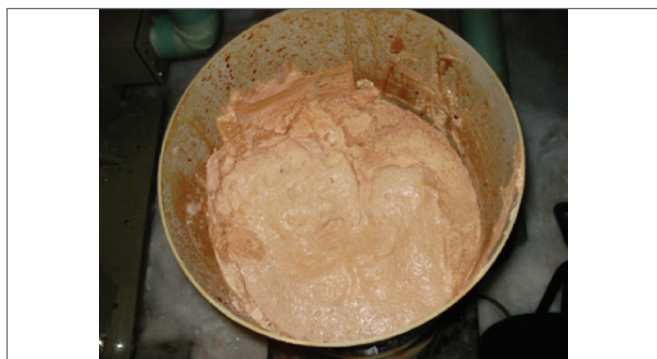
Figure 7. Elemental sulphur obtained in the liquid redox process
