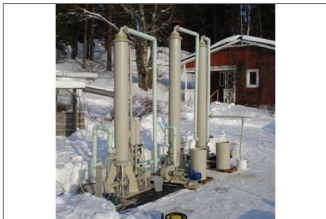
Figure 6. Test run with pilot stripping and liquid redox plant
