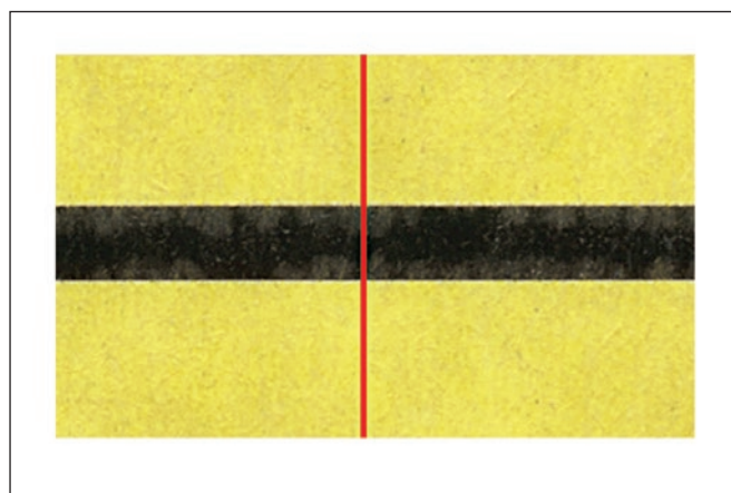
Figure 1a. The scan is taken along the red line. Any transfer of the yellow ink into the black line will be captured
