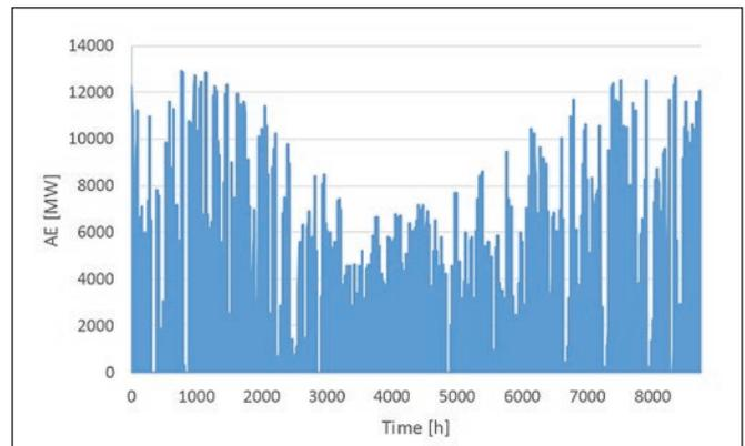
Figure 3. AE output profile along a typical year
