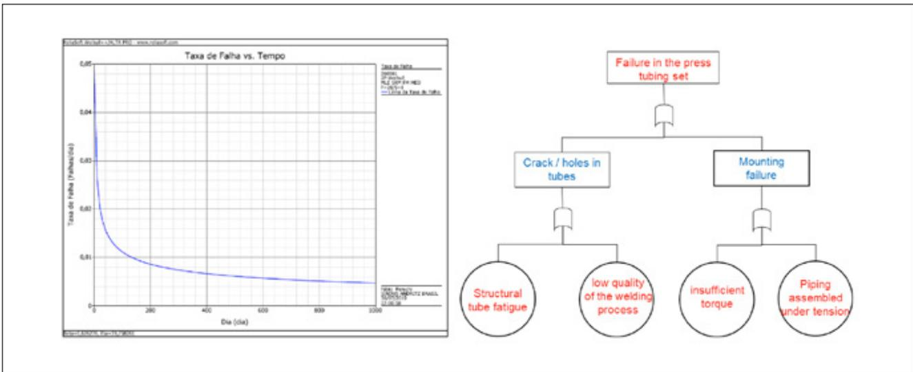
**BALE PRESS:** The behavior of the failure rate as a function of the time of the hydraulic cylinder set is shown in Figure 9, the failure rate is decreasing as a function of time (initial portion of the bathtub curve). As verified in the FTA, the failures of the press cylinders are strongly associated with the repair carried out at external suppliers and the detachment of rod fasteners.
