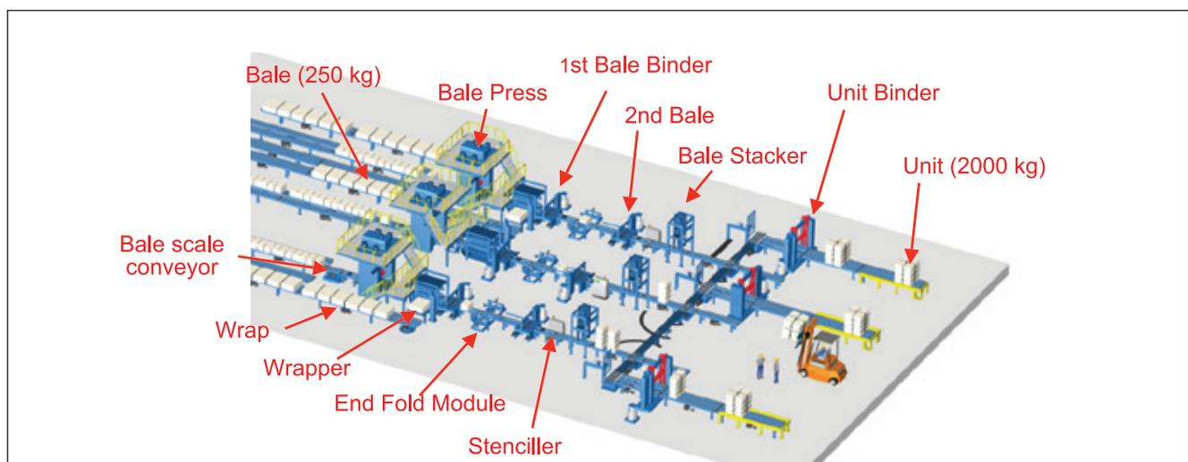
**Figure 1.** Baling Line layout
