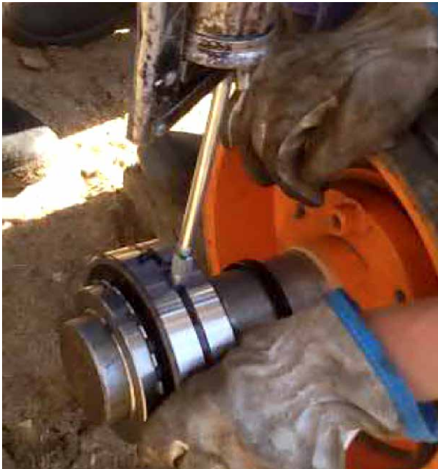
Figure 8. Grease added inside the sealed bearing
