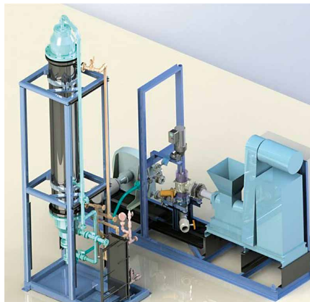
Figure 4: Design of pilot-scale continuous CNC reactor
