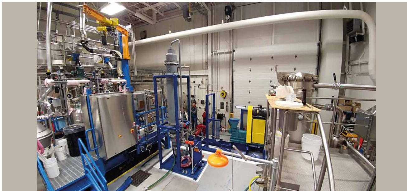
Figure 7. Integration of reactor (center) at the Innotech Alberta Inc. CNC Pilot Plant
