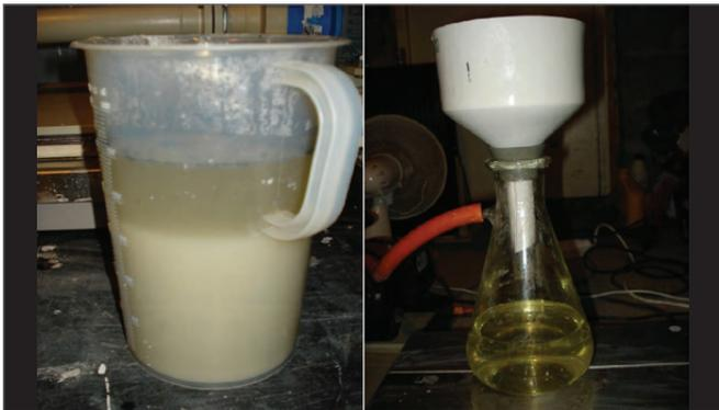
Figure 10. Product crystals, sedimenting
