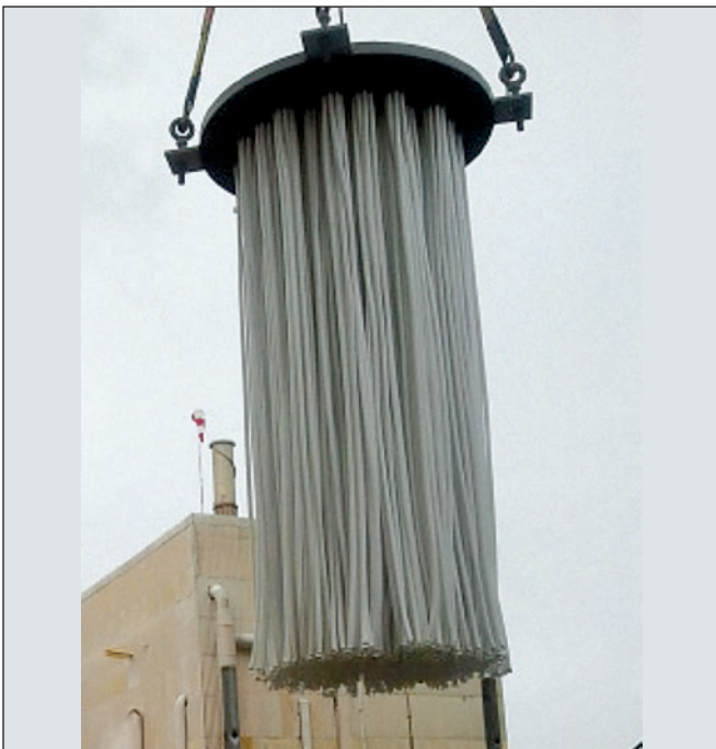
Figure 7. Pulse Filter sock assembly at Arauco Constitución mill
