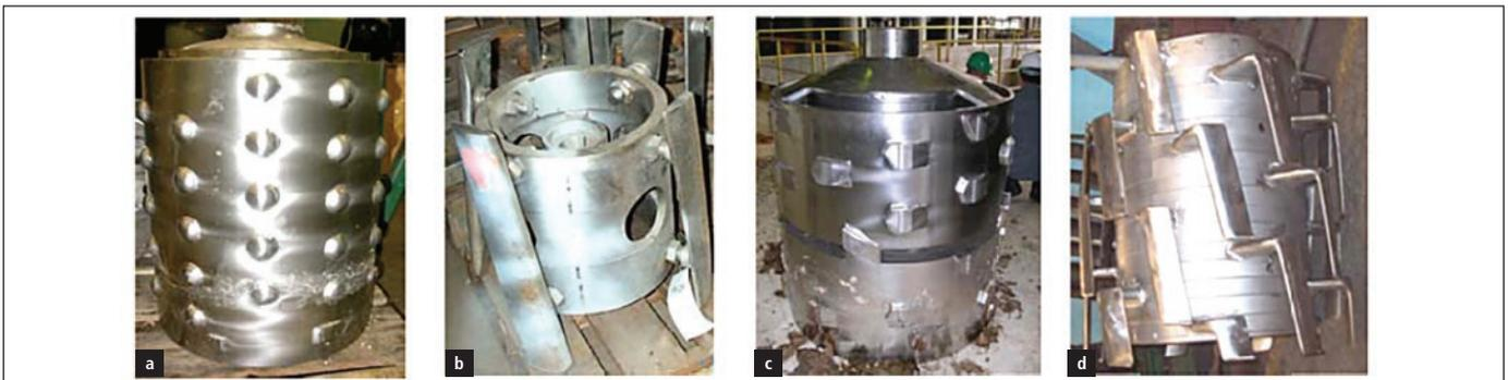
**Figure 1.** Some different rotor designs have come into use since pressure screens were introduced in the 1960s including the: a) "bump-type" rotor (1960s), b) "stud-and-nut" foil rotor (1970s), c) "modified bump" rotor (1990s), and d) cantilever foil rotor (2000's)
