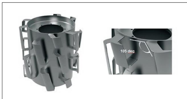
**Figure 8.** A novel, foil-type rotor (above left), features swept foils and support arms (above right) ensure there are no sites for strings or other debris to accumulate
