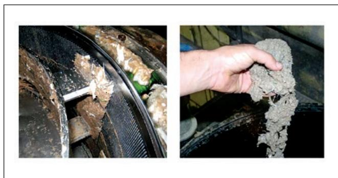
**Figure 7.** Stringy contaminants can hang up on the rotor foils and form into larger clumps which have the potential to jam between the cylinder and rotor
