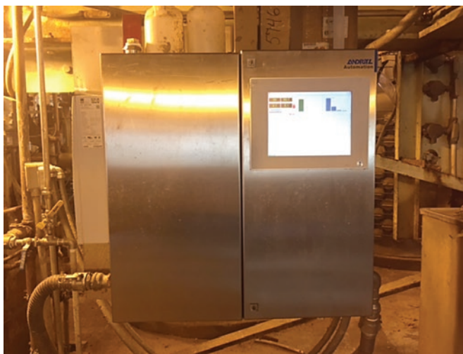
Figure 1. The in-line analyzer installed in an OCC plant
