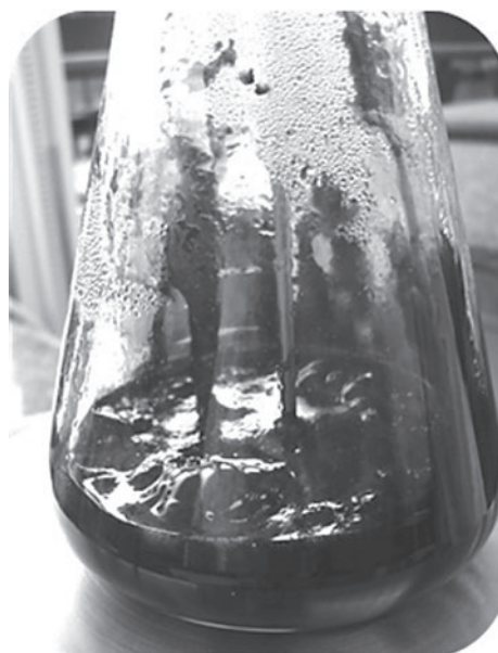
Figure 2. Boiling black liquor
