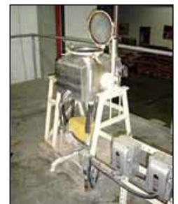
**Figure 2.** The laboratory hydropulper
