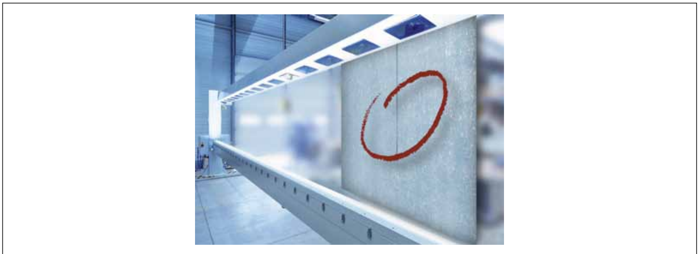
Image 4. Making invisible defects visible with the linkage of web break monitoring and web inspection systems
