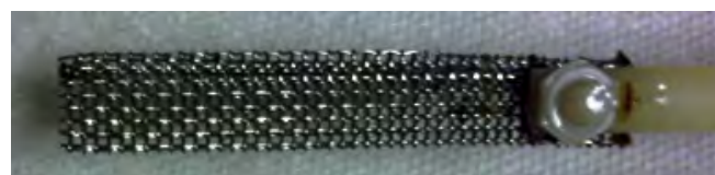
Figure 5. Mesh coupon after 30 days of BAC dosage and elimination of chlorine dioxide
