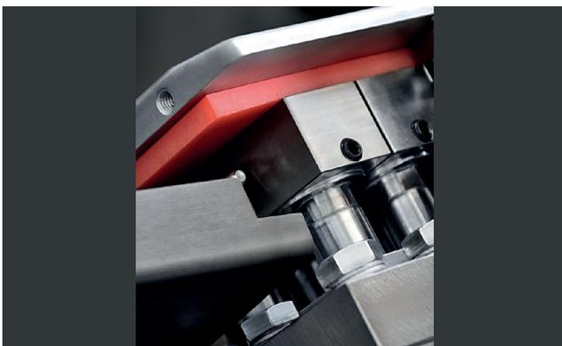
Fig. 4 – Shoe loading pistons
