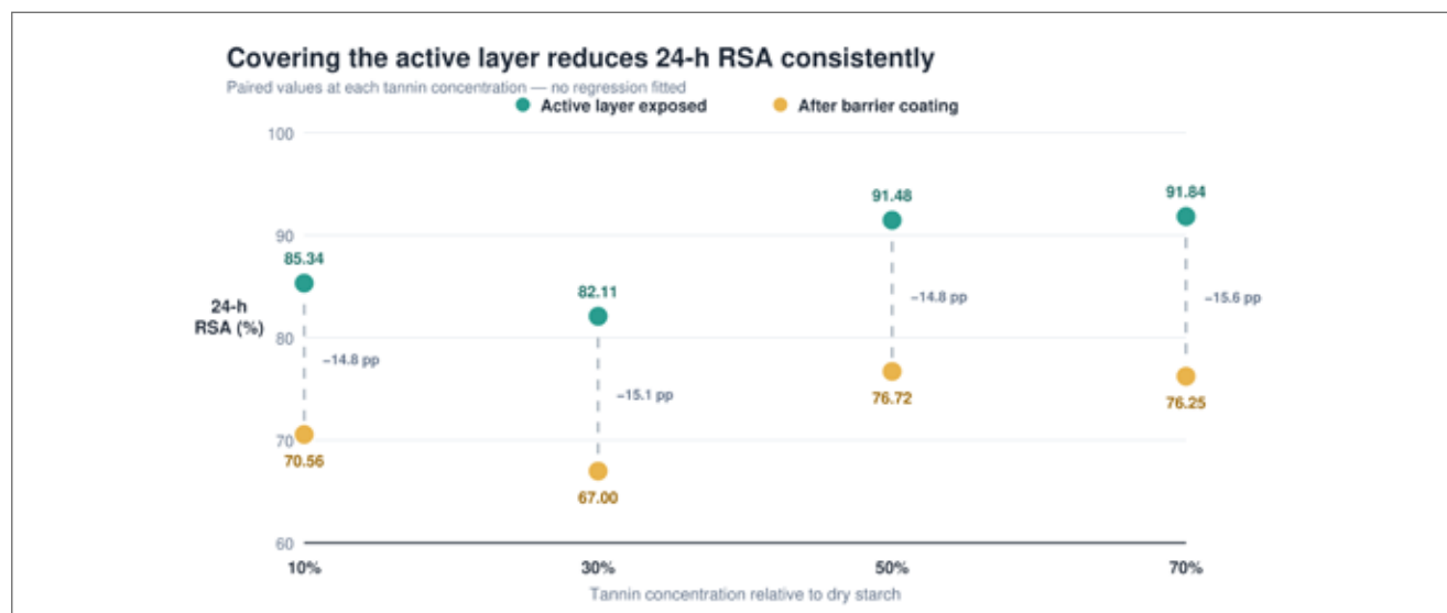
Figure 3. Twenty-four-hour radical scavenging activity (RSA) for Design I active layers containing 10, 30, 50, or 70 wt% tannin relative to starch, before and after application of the starch-beeswax barrier coating. Paired lines show the consistent decrease at each tannin concentration
